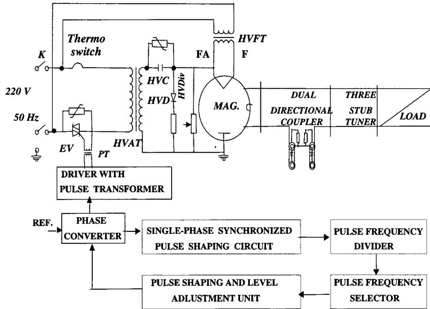
Fig. 1. Block diagram of the manual control system.
