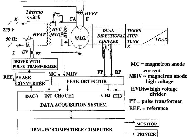
Fig. 2. Block diagram of the PC-based control system.
