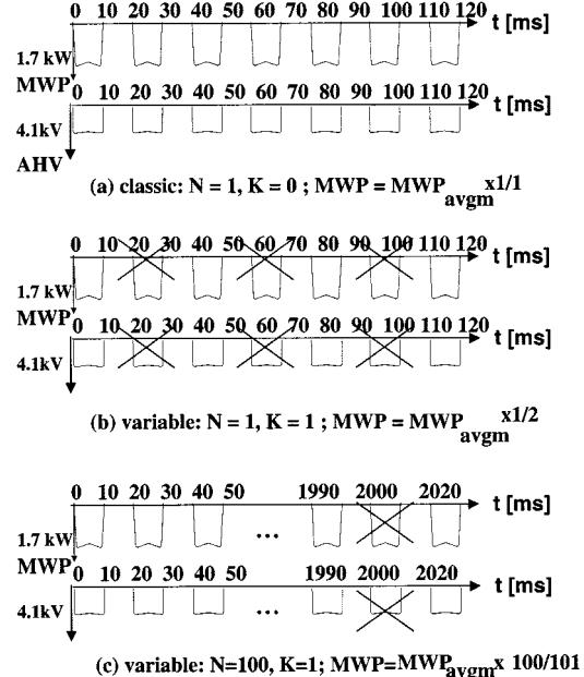
Fig. 3. Representation of the control method principle. (a) Conventional operation (no anode high-voltage pulse inhibition). (b)–(c) Anode high-voltage pulse inhibition occurs.
